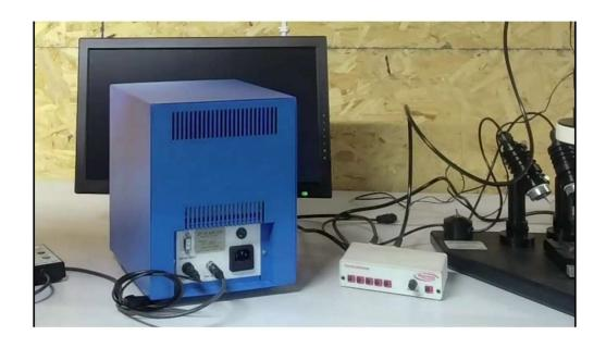
Connect temperature probe to back of instrument.
