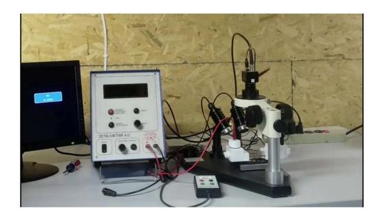
Place cell on to cell holder, connect red lead to instrument and electrode on left, connect black lead to instrument and electrode on right. You can also raise instrument bail on bottom to angle unit or can leave flat and place monitor on top to reduce space required.
