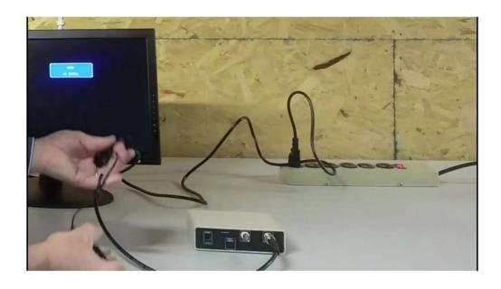
Remove the pattern generator from its box and connect the BNC cable from the monitor to the pattern generator connector marked output.
