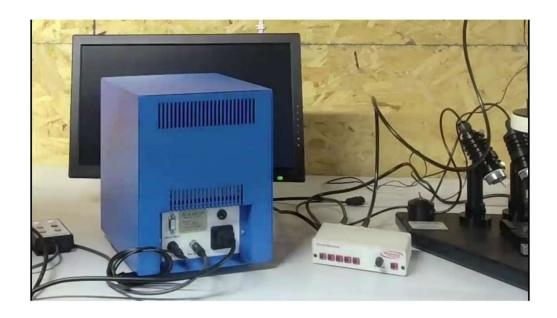
Connect power cord to back of instrument and then to power strip.
