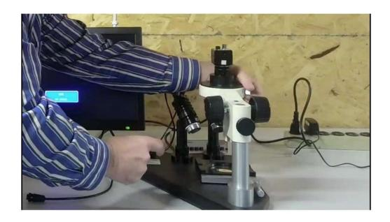
Unwrap camera assembly and place ring into holder on base. Align so camera has power on left and BNC on right. Then tighten thumb screw.
