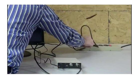
Remove the pattern generator power supply adapter and connect it to the pattern generator and power strip.
