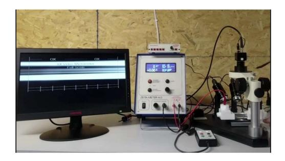
This shows the right light on and aligning the cell edge with the OX line. The line on the side of the adjustable holder gets you very close to the focus you need to get started.
