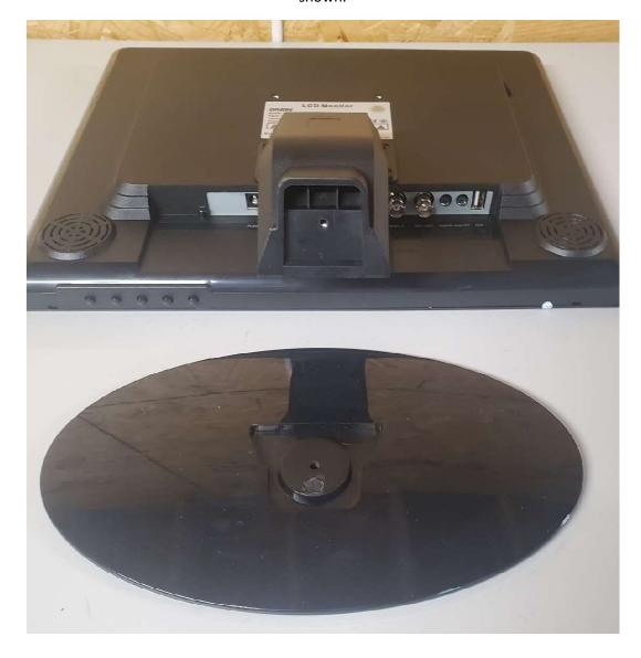
Attach the power cord into the receptacle on your left. Remove one of the BNC cables from the pattern generator box. Attache to the BNC connector toward the middle marked "BNC-1".
