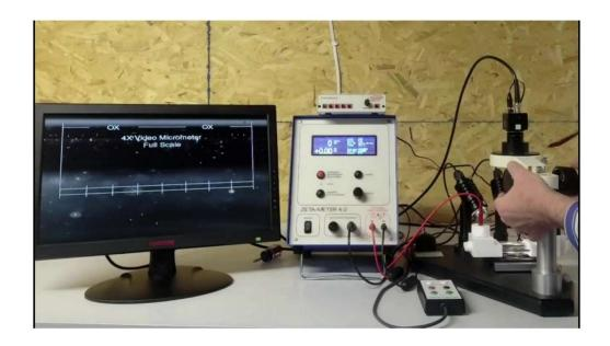
This shows particles in the fluid. You may need to adjust up and down to get better focus on particals.
