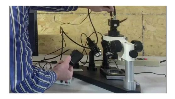
Connect camera power supply to camera and power strip.
