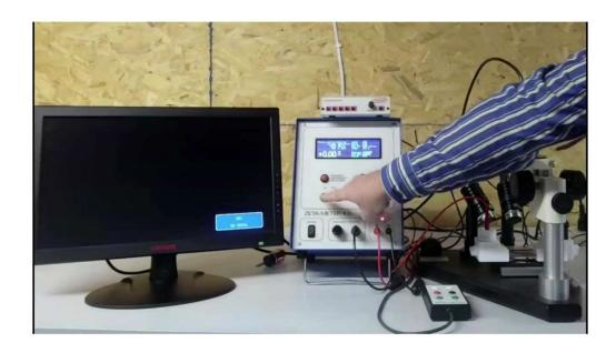
Connect light cable from base to instrument. You can now run a specific conductance test to make sure everything is working. It will be zero as you have no fluid in the cell yet.
