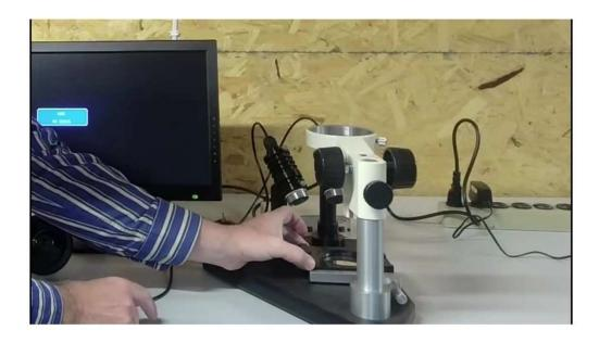
Remove base from box and place in front. Place the mirrored cell holder onto base with the holes going over the two post on the base plate.
