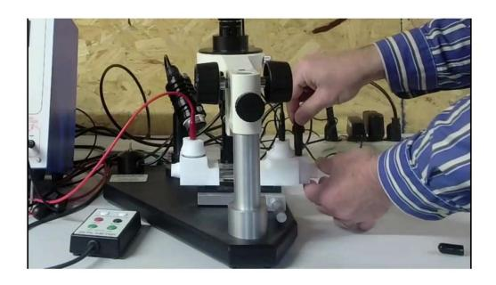
Place temperature probe into opening in cell.
