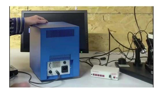
Connect keypad to back of instrument.
