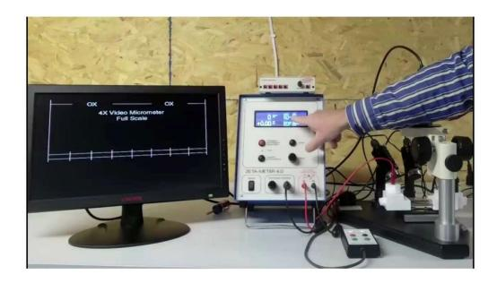
You want to make sure you are measuring the correct distance. This shows the pattern generator is set to full scale.
